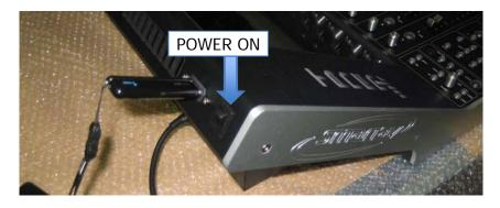
To switch the power off, select the "System" menu tab on the LHS of the display. Then select "Shutdown" from the system menu and "Confirm". The console will take several seconds to shutdown from this point.
