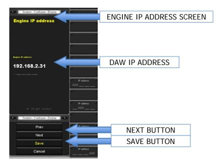
• Use the knobs on the RHS of the screen to enter the IP address of your Logic MAC. This is the IP address assigned to your DAW in the "Network Connection" section of this manual.
